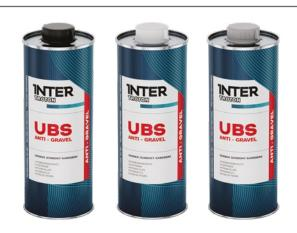
Product based on synthetic resin designed to protect car bodies from the harmful effects of gasoline, oil, water and salt. Creates a strong and flexible layer for maximum stone chip protection. Features sound-absorbing and soundproofing properties. It does not contain asphalt and bitumen. Can be over coated with any acrylic lacquer. Product efficiency for 1 liter: about  $3,5\text{m}^2$  of dry layer with total thickness of  $100\mu\text{m}$ .
