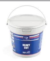
S07 polishing paste of the highest cutting level can be used on a mold or products made of industry gelcoat. It removes the deepest defects made during grinding with P800 paper. The paste does not contain silicone or wax fillers.
