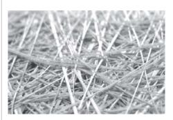
Glass fiber mat, in connection with laminating resin, is used for the repairs of big holes in boats, yachts, camping caravans, etc. The repaired elements may be made from steel, aluminum or GRP, reinforced with glass fiber. The obtained layers have very good adherence, are durable, resistant to petrol, oils, greases, and the short period temperatures up to 70°C.
