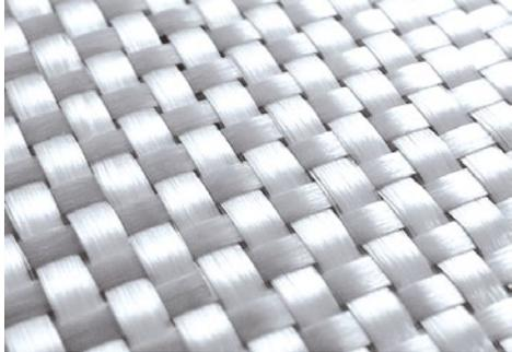
Woven roving fabrics work as a reinforcement for polyester resin in the production of laminates. They offer a higher amount of glass content significantly increasing the strength and durability of the laminate, especially along the roving strands. Available in gradations of 150, 200 and 400 g / 1m<sup>2</sup>.
