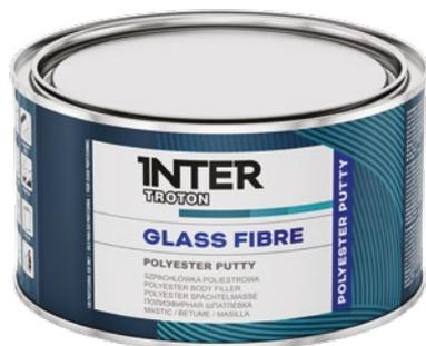
Body filler reinforced with glass fibre, dedicated for filling large dents and holes in vehicles, caravans and trailers. Provides high structural strength with good elasticity and sanding properties. Ideal for deep filling application on small surfaces.
